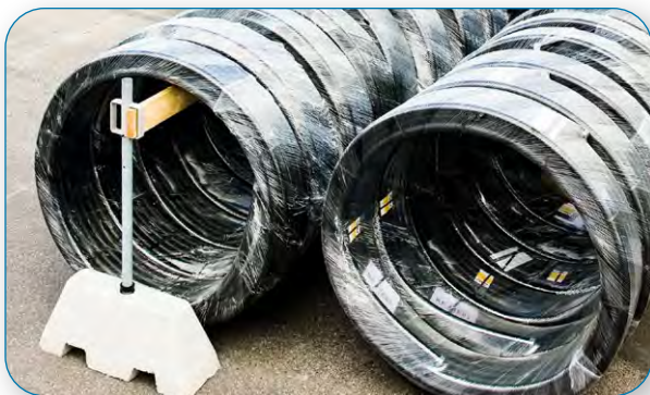
When coils are stored upright they need to be supported to avoid deformation of the pipe.
