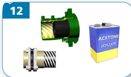
12 Clean the scraped area on the transition fitting and inside of the termination fitting with acetone or isopropanol.
