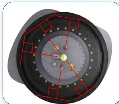
Make sure the pipes are in a straight angle to the chamber wall and fittings on the manway lid.
