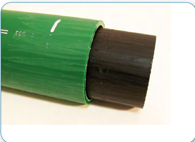
Insufficient scraping. Not all areas have been scraped.
