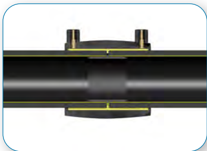
Pipes must be cut squarely to fit the welding socket.
